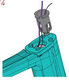
Route Di2 cable & brake hose through the largest hole in the compression nut.
