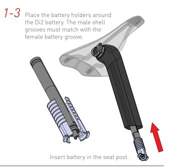
and use to guide the seat post wedge into position
