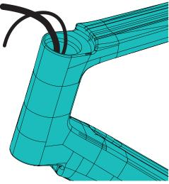
Route the Di2 Shifter cable from the Junction B through the down tube, until it exits the head tube.
