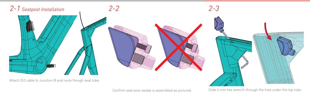
Secure the seat post by tightening the M8 grub
