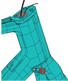
Secure the headset adjustment by tightening the M5 Ti screw to 4 Nm.
