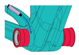
Install the provided Wheels MFG BBRight adapters if using cranks with a 24mm spindle.
