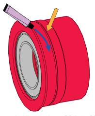
Clean the inside of the frame BB & the BB cups with isopropyl alcohol. Apply Loctite 641 on the grooves of the both BB cups.
