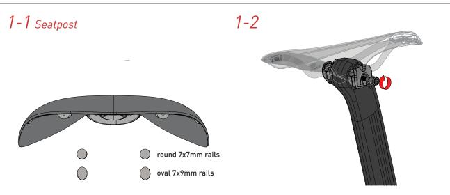
Adjust the set back and saddle angle to the desired position. Tighten the M6 saddle clamp bolt to **12 Nm.**
