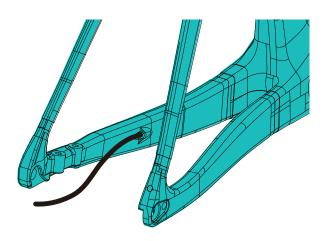
Cut the cable housing to the correct length
