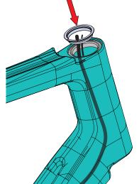
Lightly grease and install headset compression ring.
