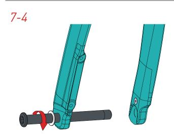
Remove the thru-axle and remove the hub. Install front wheel and tighten the thru axle (with the nylon washer) to **12Nm.**
