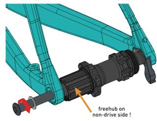
6-3 After ensuring the dropout insert is correctly aligned, tighten the dropout bolt to 1 Nm.
