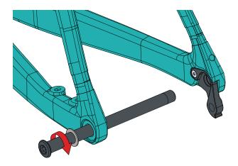
Remove the thru-axle and remove the hub. Install the rear wheel and tighten the thru-axle (with the nylon washer) to 12Nm.
