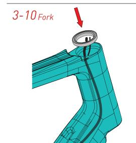
Lightly grease and install upper headset bearing as pictured
