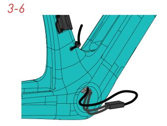
Route the front derailleur Di2 cable through the seat tube hole to the bottom bracket exit port.
