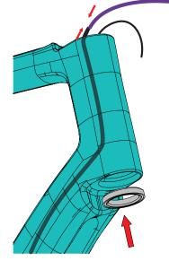
Lightly grease and install lower headset bearing.
