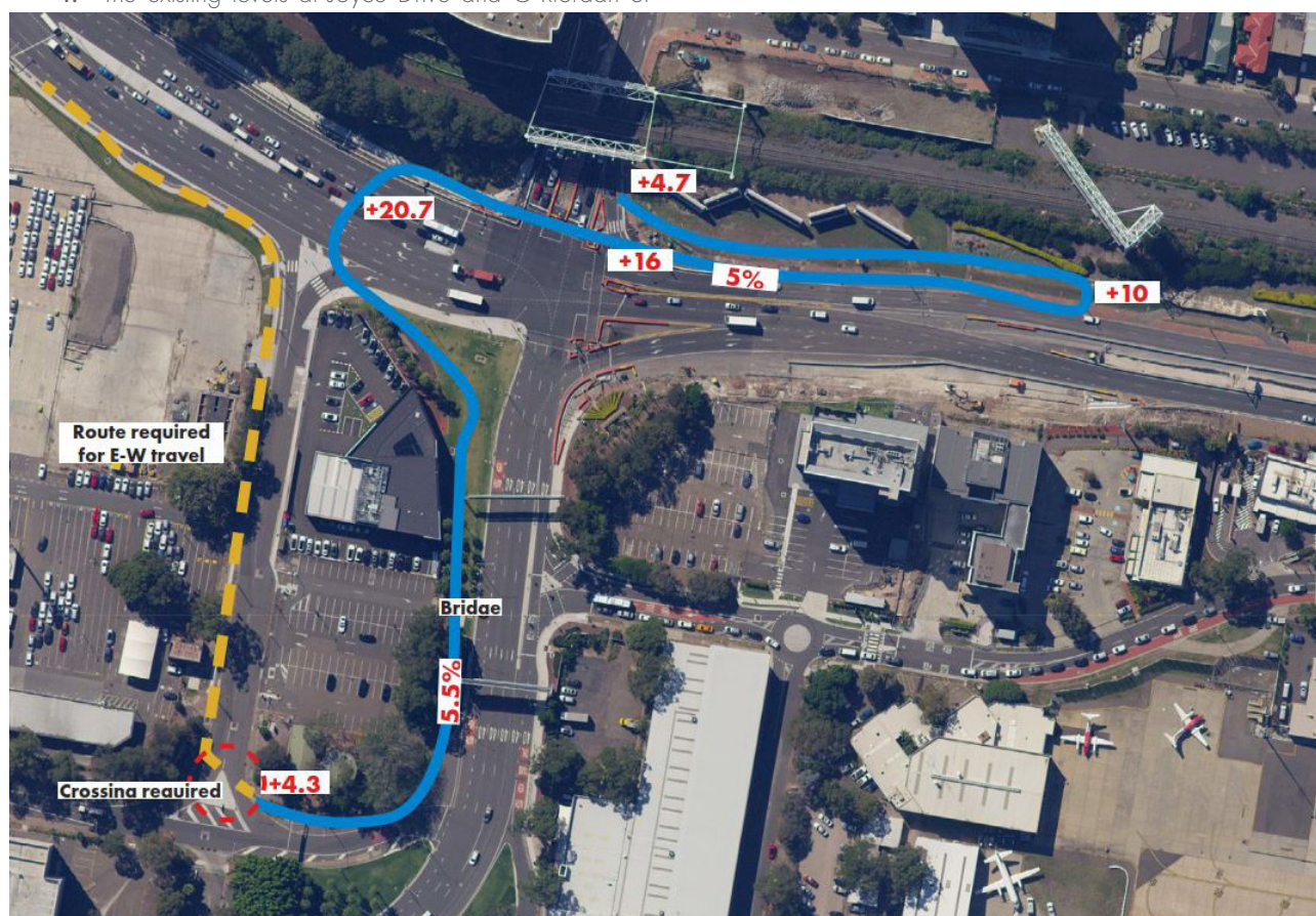
Figure 22: Overview Joyce Drive overpass
