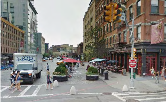
Curb extension marked by bollards and paint, location unknown, image by Google Earth
