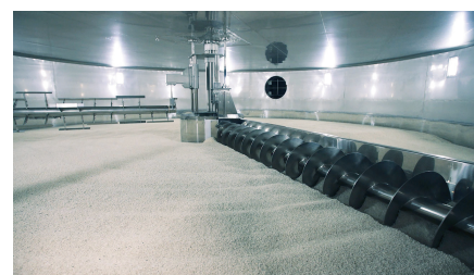
Rotary Type Automatic Koji Making Equipment (inside) From heaping to discharging, this rotary automatic system enables fully automated, unmanned operation. By maintaining optimal temperature and humidity, it ensures the production of high-quality koji.
