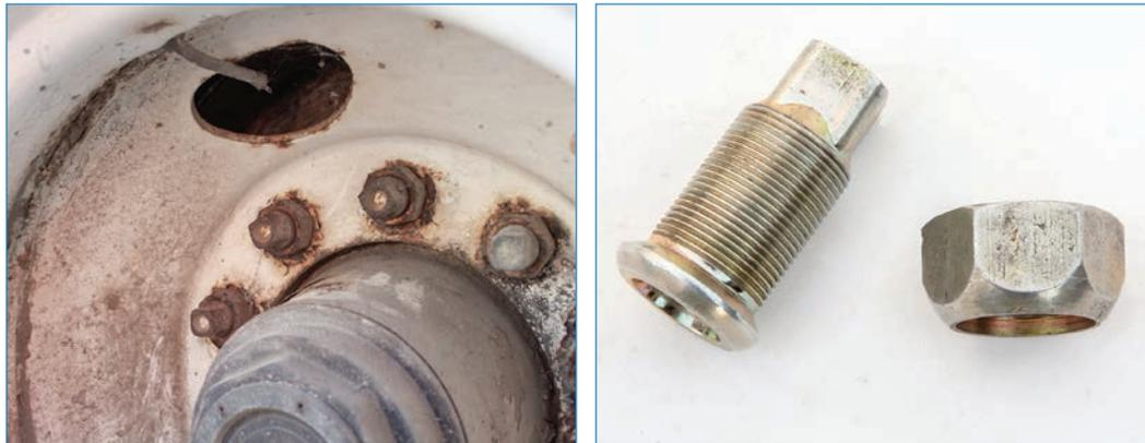
**Hub piloted** — This mounting system uses the centre or hub of the wheel to carry the weight and align it properly. The holes in these rims for the studs to go through are flat and the wheel nuts used come with a built-in flange washer, so the nut doesn't dig into the rim when you're tightening it up.
