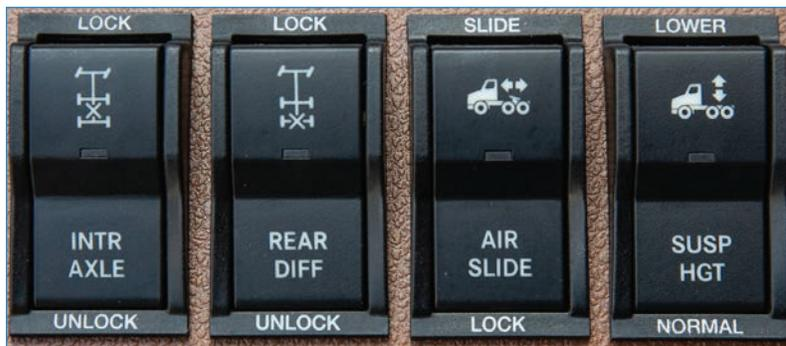
**Differential (Diff) lock** — Also called “main differential lock” or “driver controlled differential lock” (DCDL). This locks both sets of dual wheels on the same axle to ensure they both spin together at the same speed. It should be used when operating on slippery or uneven surfaces.
