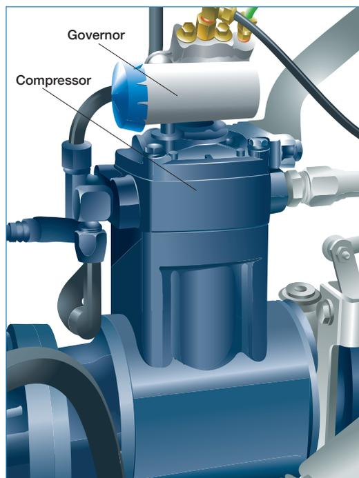
The compressor is usually mounted on the engine of an air brake-equipped vehicle — on most, it's mounted on the side of the engine and driven by gears. A belt, like a fan belt, drives some compressors on older and smaller vehicles. As long as the engine is running, the compressor will be running. The compressor must be able to build air pressure from 50 p.s.i. (350 kPa) to 90 p.s.i. (620 kPa) in under 3 minutes.
