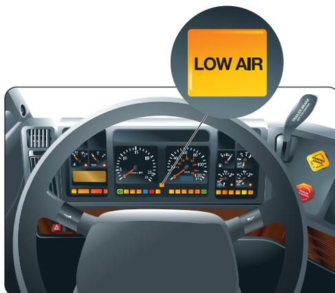
The low air warning device should come on when air pressure drops below 60 p.s.i. (414 kPa).
