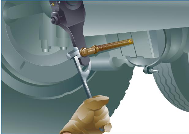
In the diagram, the driver is pulling on an air brake slack adjuster to measure if the brake is within adjustment tolerance.
