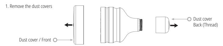
PBM dust covers for the 25 mm adapter should be wiped down with Caviwipes or equivalent product to avoid potential cross contamination.
