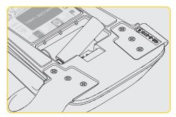
Install the provided 2 AA batteries
