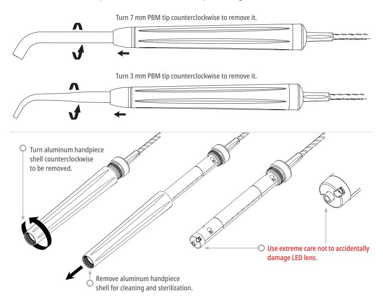
To reassemble, slide the handpiece shell onto the handpiece body and turn clockwise to tighten.
