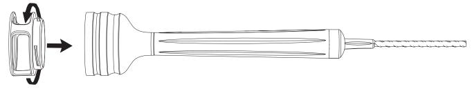
The PBM adapter is now ready to use. To remove the PBM adapter, unscrew it from the Gemini EVO laser handpiece, remove and discard the spacer, and re-install dust covers when not in use.
