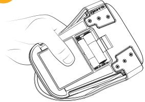
Keep the pedal depressed. Install the 2 batteries and keep the pedal depressed for 15 seconds.
