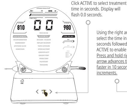
Using the right arrow select the time in seconds followed by ACTIVE to enable timer. Press and hold right arrow advances timer faster in 10 seconds increments.
