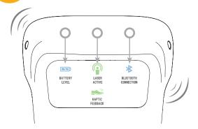
Activation Pedal icons will flash simultaneously along with the haptic feedback indicating pairing mode sequence has started. You can now release the pedal.
