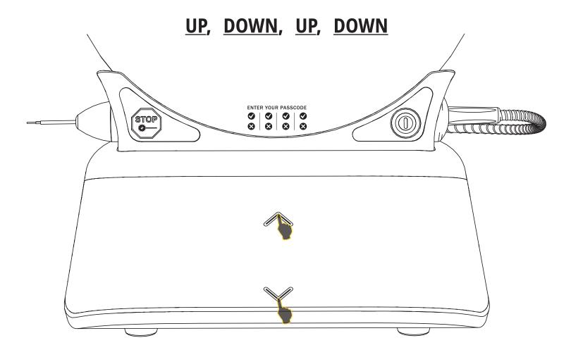
The Gemini EVO 810+980 soft tissue laser is equipped with Guided Touch Interface "GTI" which means only the icons that are relevant for a given procedure will be shown. When entering the electronic key passcode, only the UP and DOWN arrows will be shown as they are the only necessary icons to be touched while entering the passcode.
