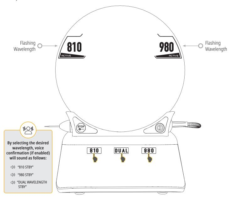
When selecting a wavelength, the 3 wavelength options 810 / DUAL / 980 will be shown as they are the only necessary icons to be touched while selecting a wavelength.
