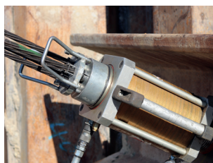
80 TO CFK SPANNPRESSE, 19KG
