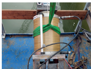
270 TO CFK SPANNPRESSE, 82KG
