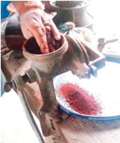
C. Grinding nodules into powder
