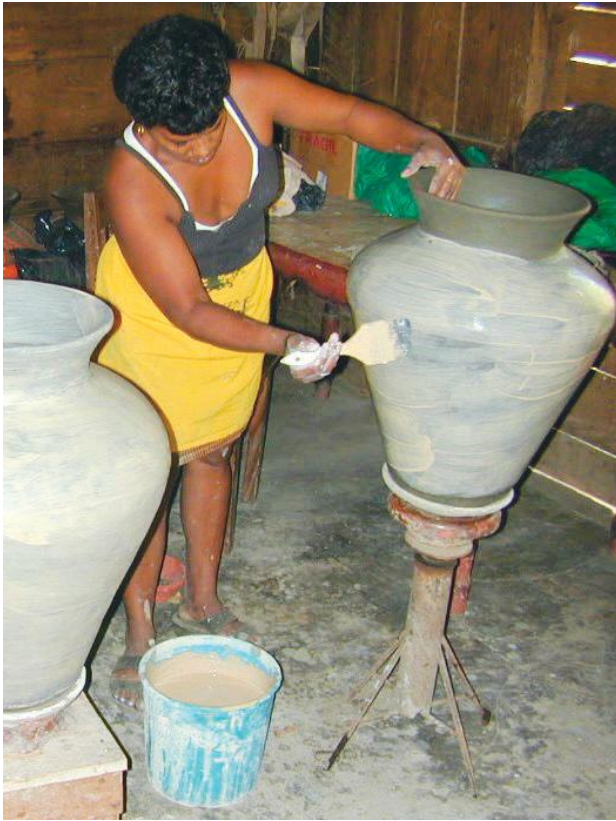
A. Applying slip ( engobe in both Engl. and Span.)
