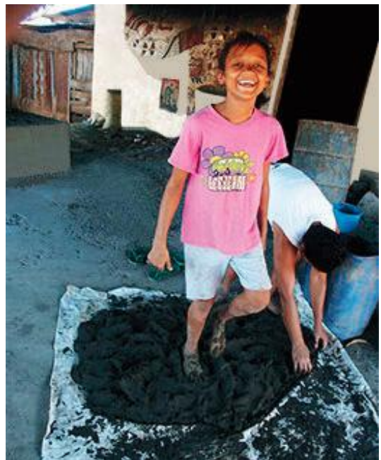
C. Mixing clay with “iguana sand” and water
