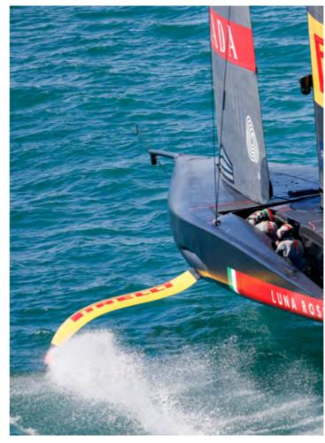
The foil adjusts to ensure that the lift always equates to the weight.
