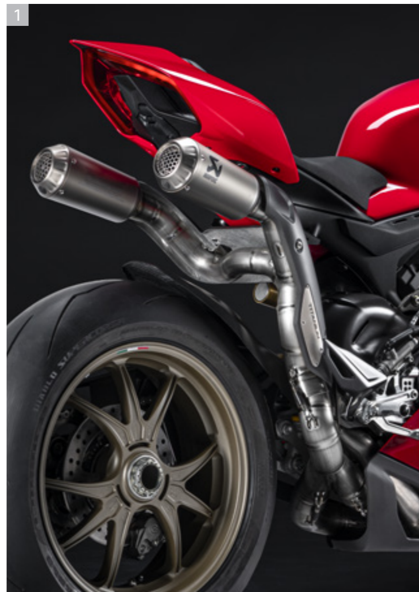
1 Complete titanium exhaust system.
