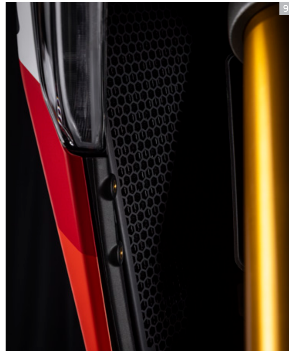
9 Aluminium protection grid for water radiator.
