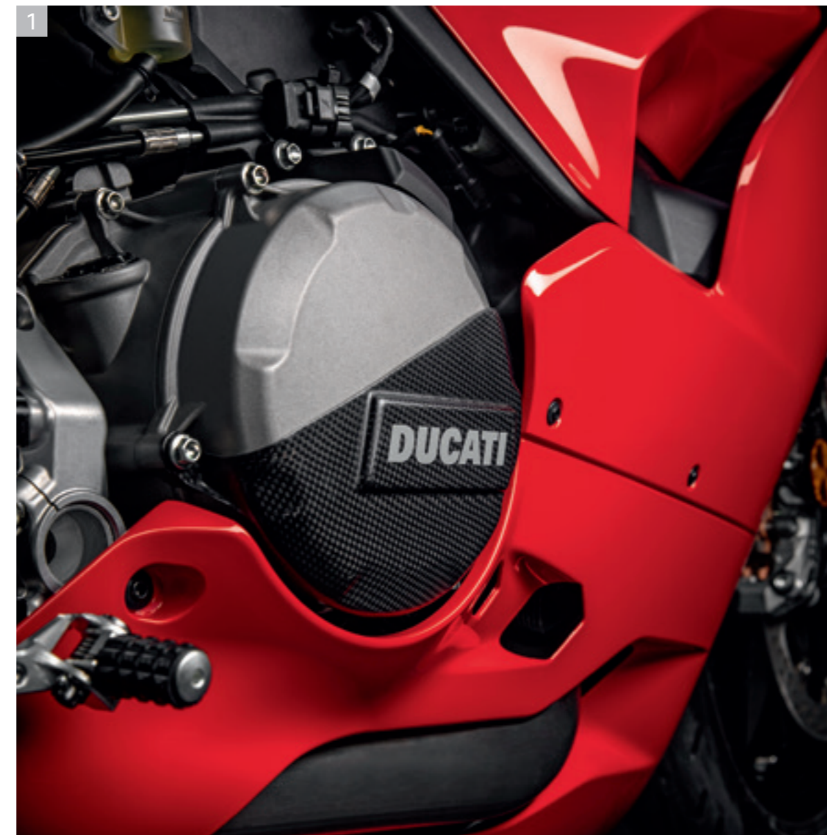
1 Carbon cover for clutch case.
