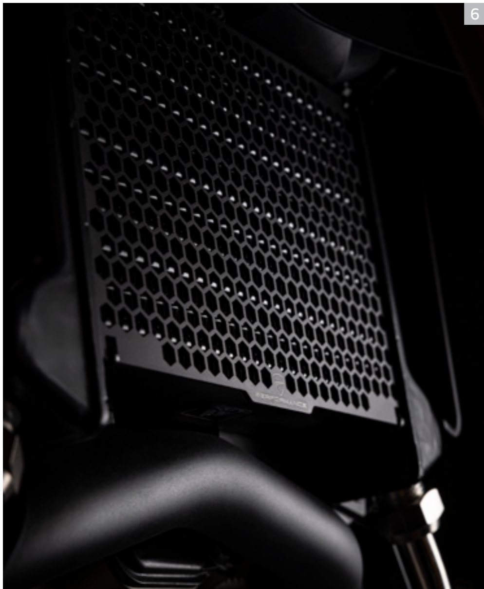
6 Aluminium protection grid for oil cooler.
