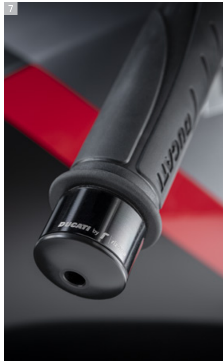
7 Billet aluminium handlebar balancing weights.
