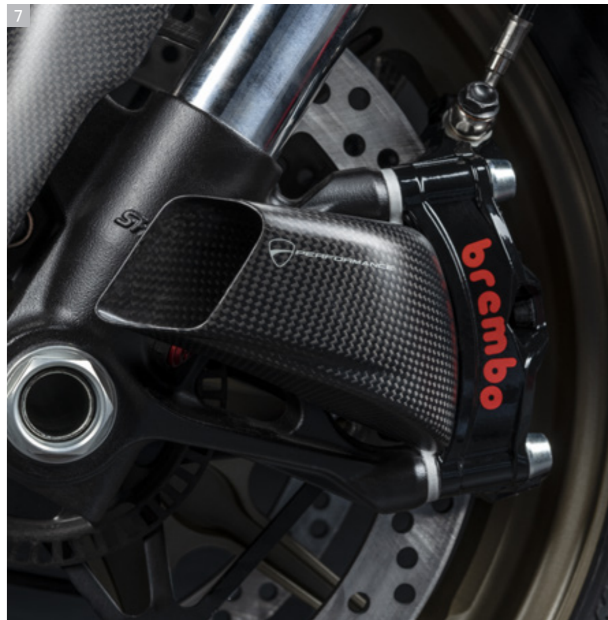
7 Carbon ducts for brake cooling. Coloured front brake callipers.
