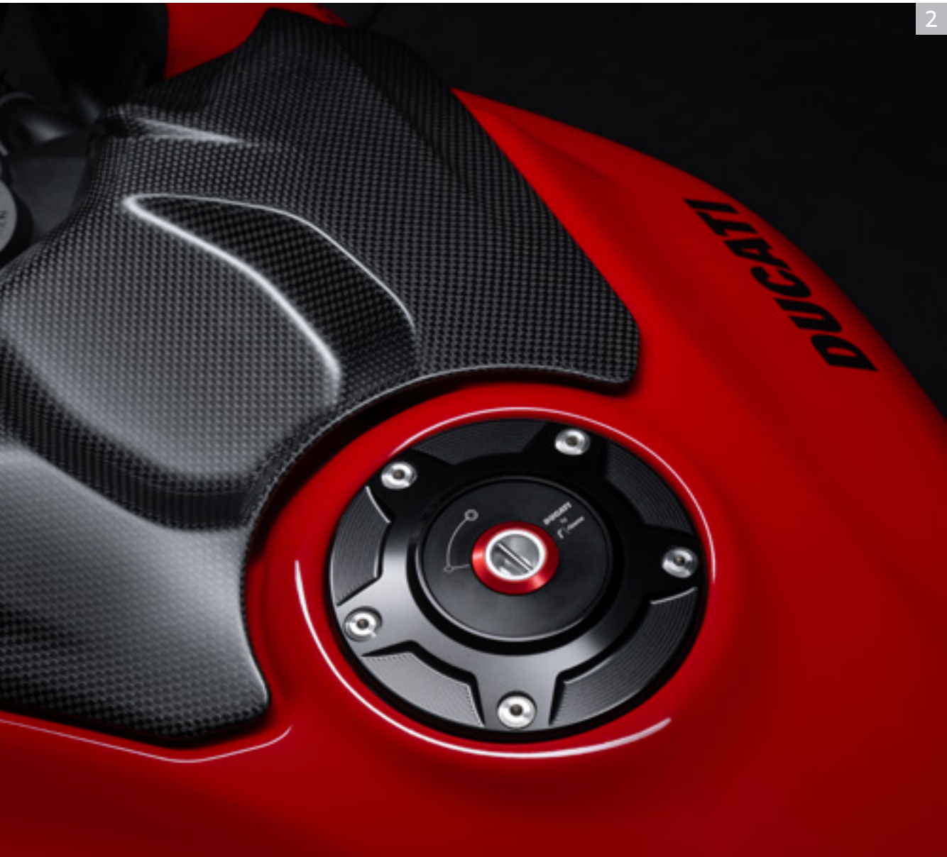
2 Carbon tank cover. Billet aluminium tank cap.
