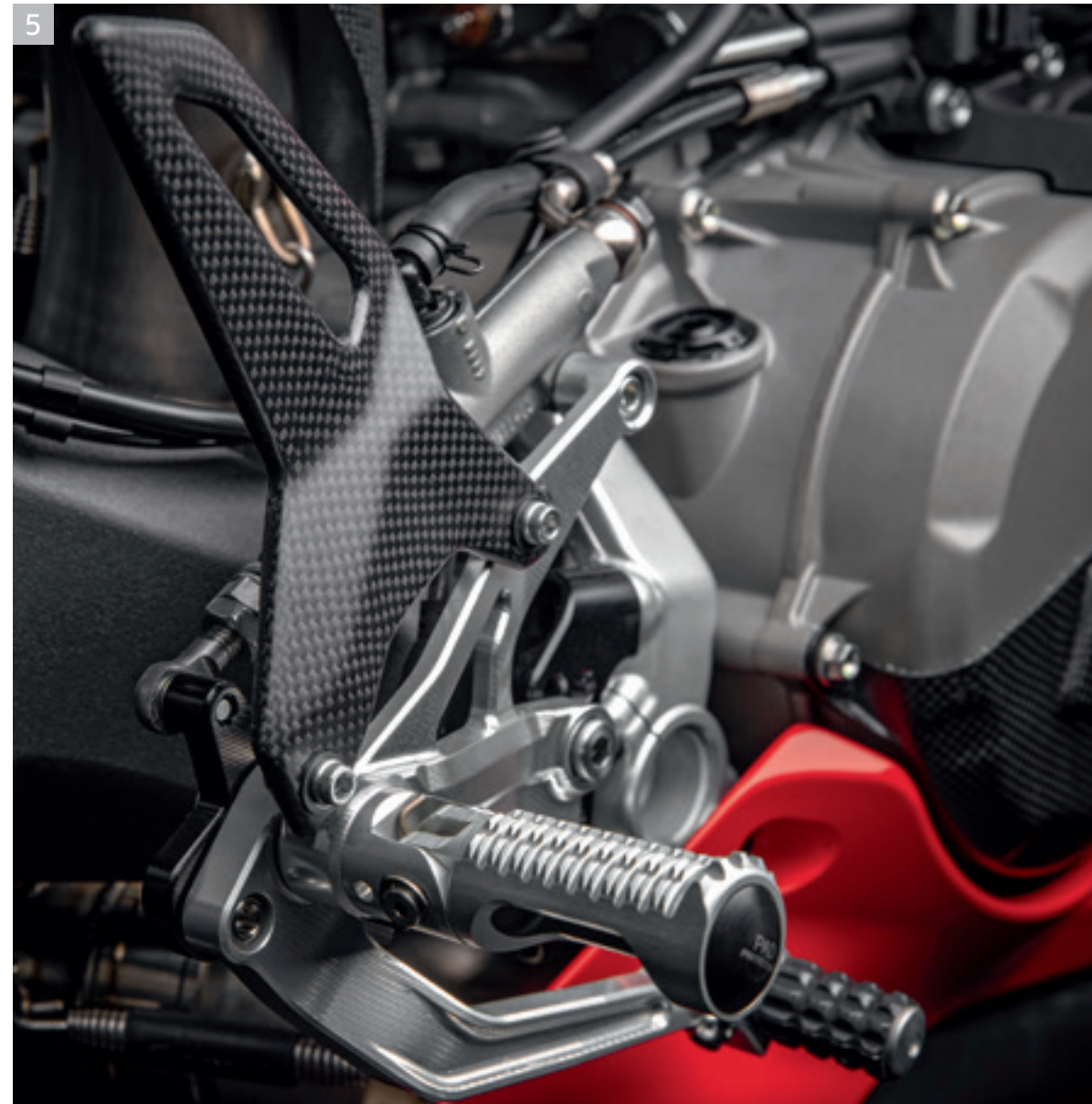
5 Carbon heel guard. Adjustable rider footpegs in aluminium.
