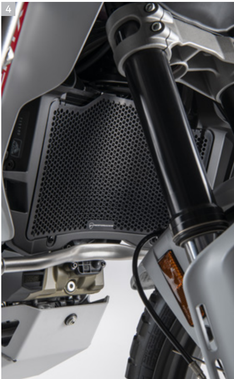
4 Protective mesh for water radiator.
