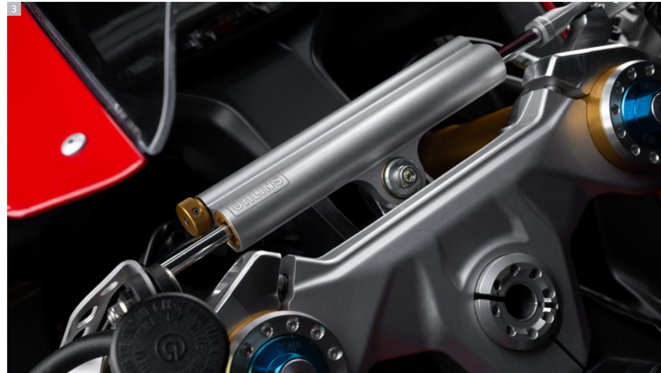
3 Öhlins adjustable steering damper.
