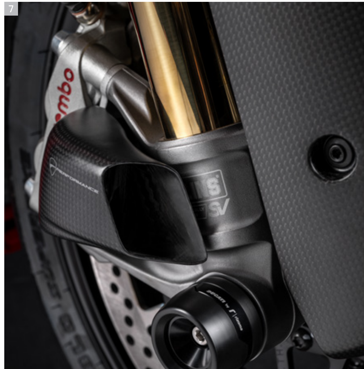
7 Carbon ducts for brake cooling.
