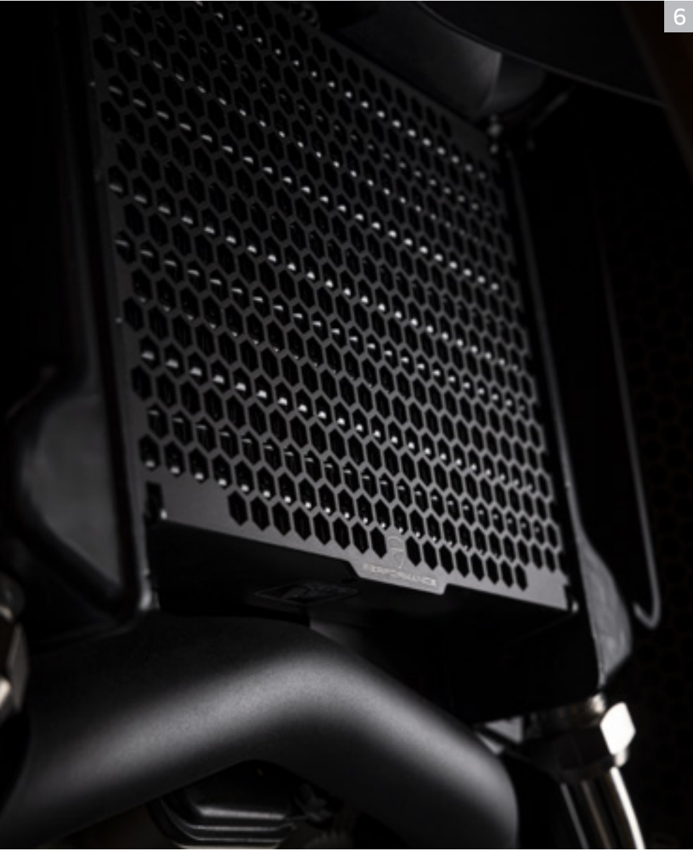
6 Aluminium protection grid for oil cooler.
