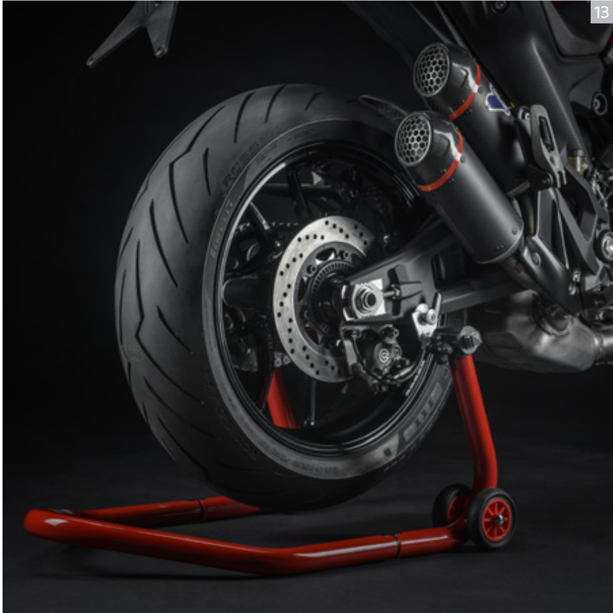
13 Rear service stand for double-sided swinging arm.
