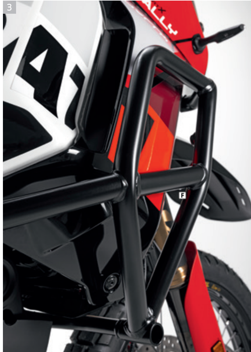
3 Engine cover in steel tubes.
