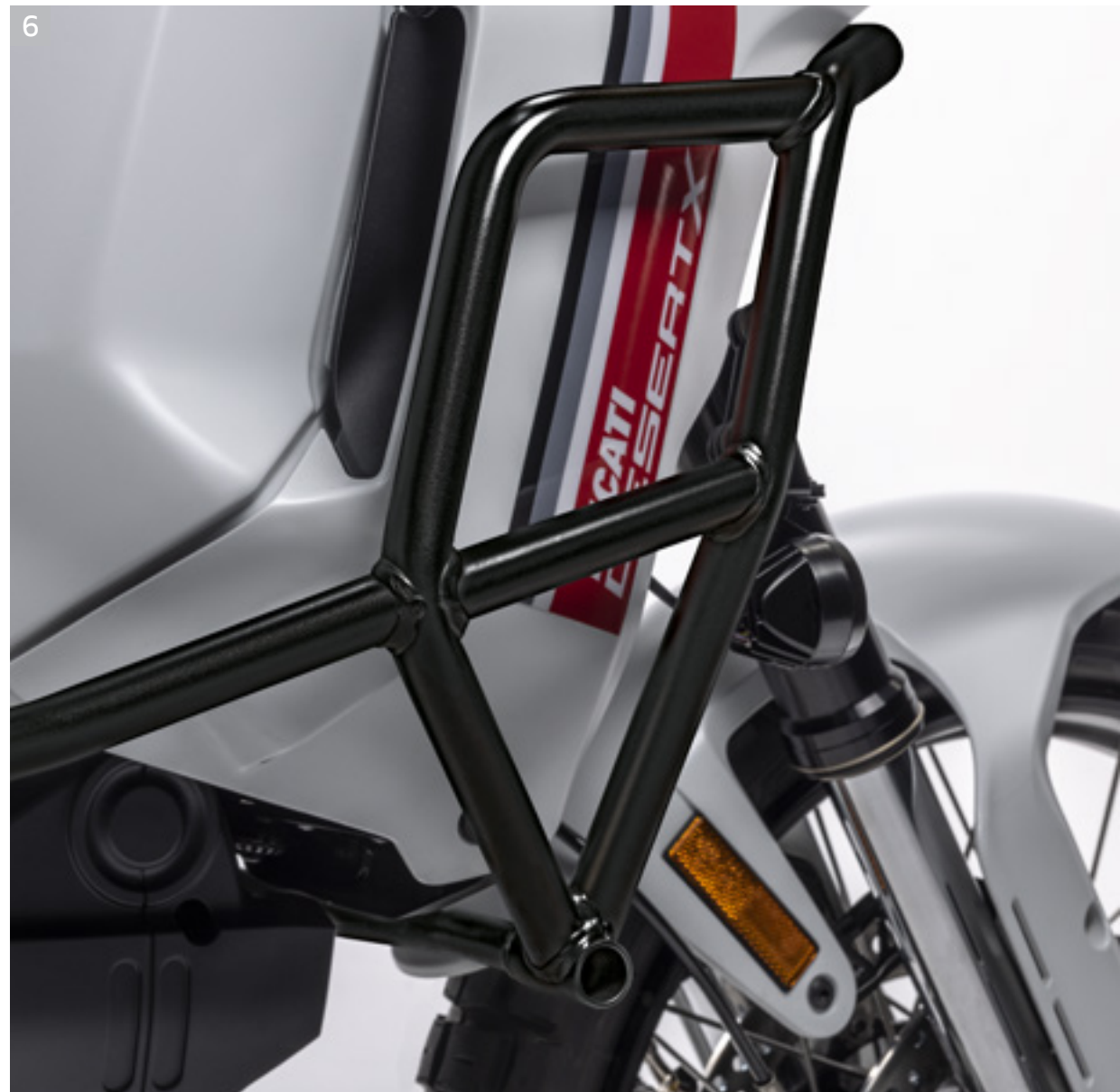
6 Engine cover in steel tubes.
