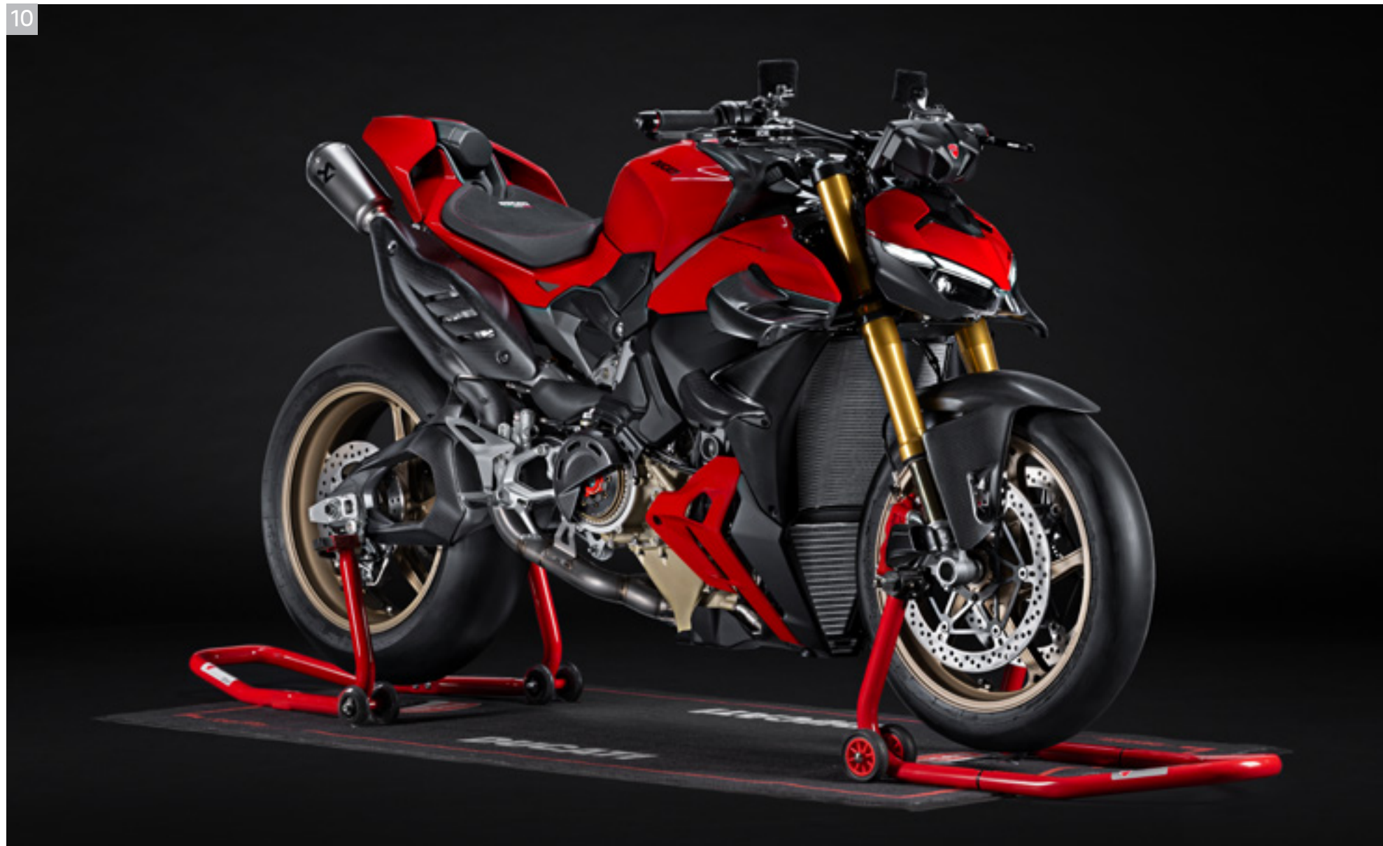
10 Garage Mat. Front service stand and rear service stand for double-sided swinging arm.
