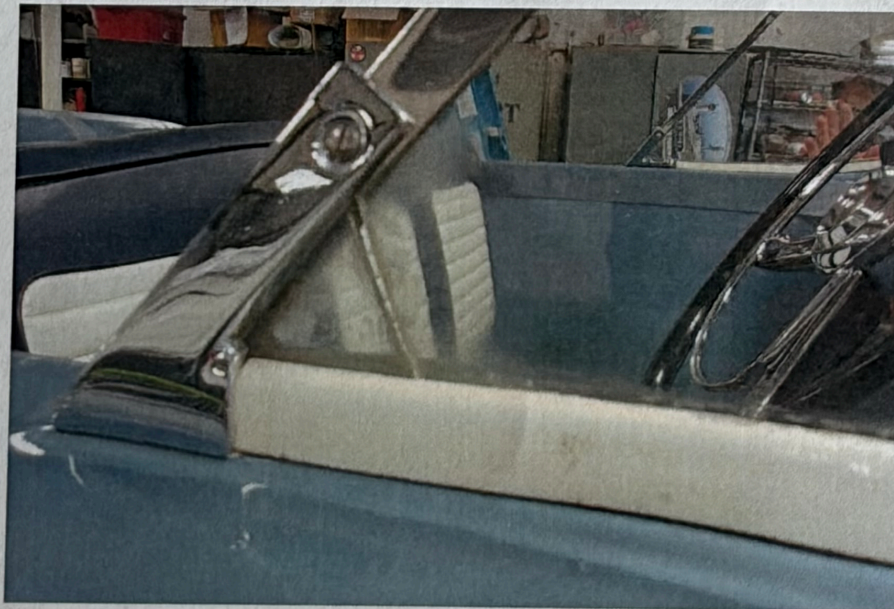
CORNER OF WINDSHIELD BROKEN
