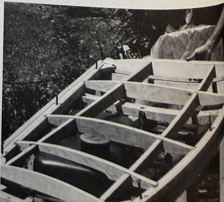
4 Ribs with varied curvature turn out just right with the paper tab method. Accuracy is essential here in order to obtain a good glue contact surface overall.
