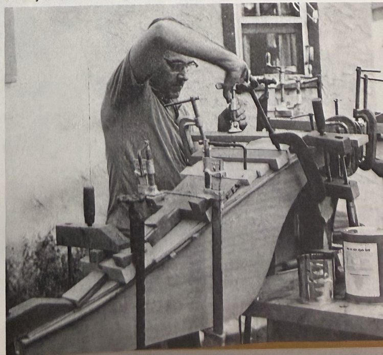
10 Sufficient clamp pressure is essential for this kind of a glue-up. Skin being glued to the kerfed section is \frac{1}{4} " marine grade mahogany veneer plywood. Waterproof glue but no nails or screws were used on any of the surfacing veneers.
