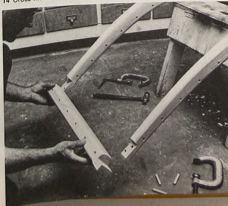
14 Cross members are joined with strong doweled lap joints.
