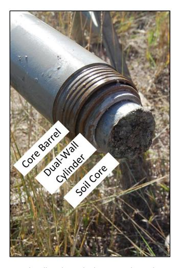
Figure S-3. Dual-wall cooling cylinder inserted into the core barrel.
