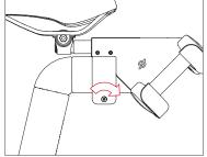
▲ WARNING: Do not over-tighten the seat slider adjustment knob. Over-tightening could result in malfunction or breakage.
