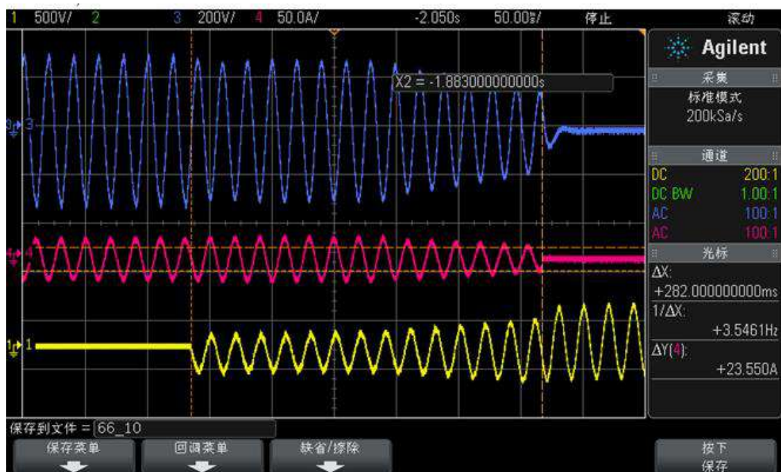
Graph of disconnection at balance condition ( P_{AC} 0 and Q_{AC} -1% reactive load) @66% nominal power
