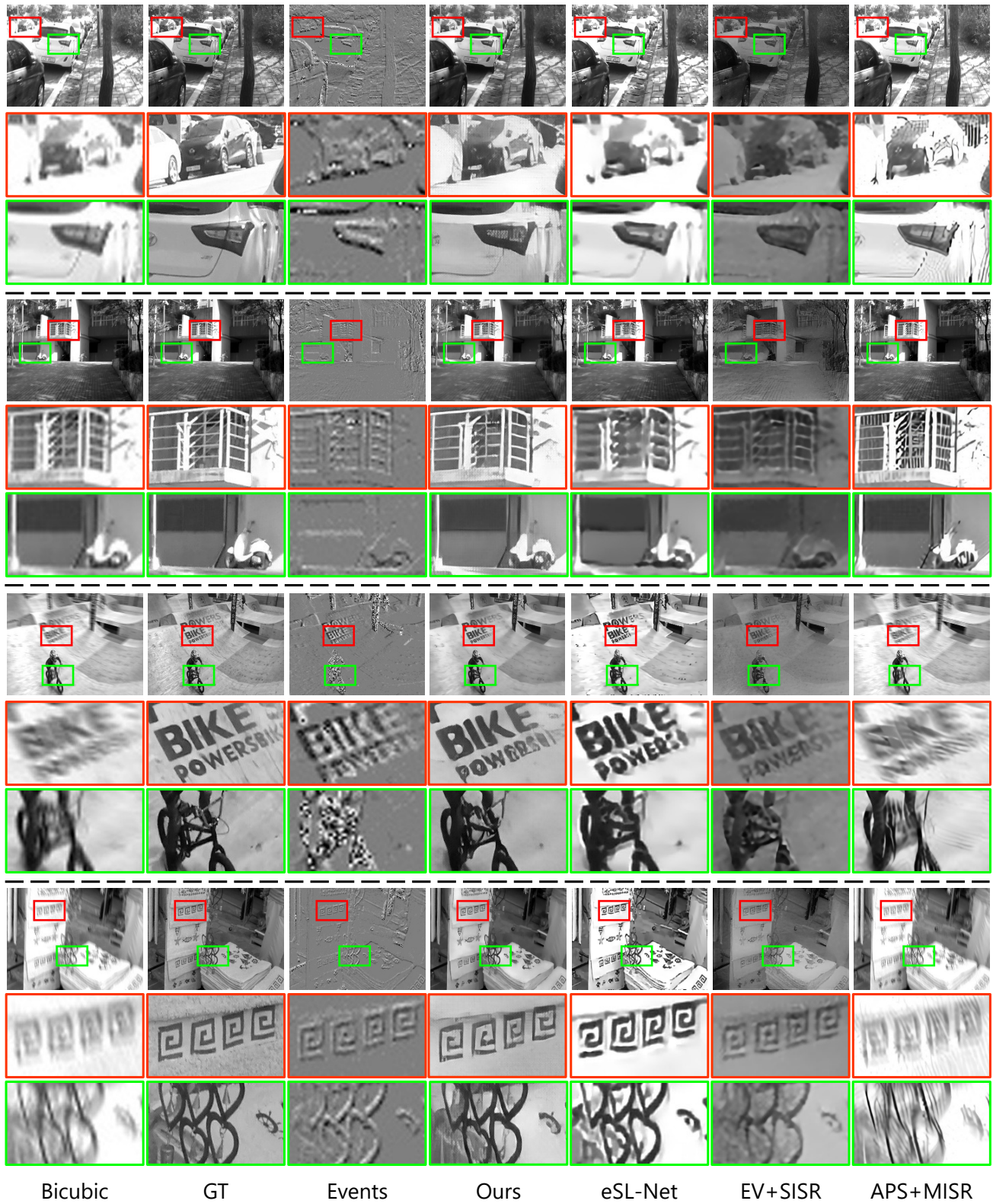
Figure 9: Visual quality comparison of 4x SR on synthetic dataset between EvIntSR-Net and other state-of-the-art super-resolution methods.
