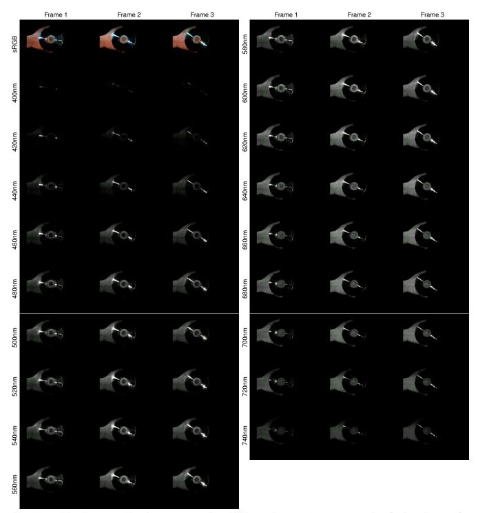
Figure 22. Real-time hyperspectral imaging on a compact disc exhibiting varying spectral responses across its reflection strip. Top-left: Three consecutive estimated hyperspectral images rendered in sRGB. Remaining panels: Corresponding estimated hyperspectral images (380-780nm, sampled at 20nm intervals).
