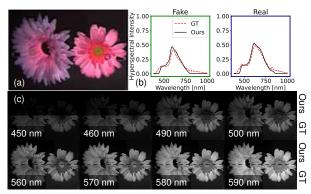
Figure 7. Evaluation on metameric samples of fake (left) and real (right) daisies. Our method achieves 10.8 SAM and 34.95 PSNR on average. (a) The reconstructed hyperspectral image in sRGB. (b) Spectra of metameric samples against ground truth measurements, highlighting the system's ability to capture subtle spectral differences. (c) Estimated hyperspectral images.
