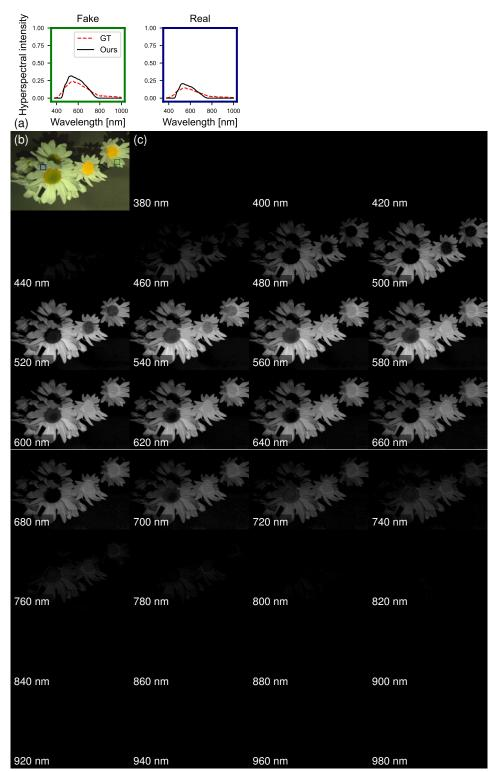
Figure 16. Evaluation of metameric samples of real (left) and fake (right) white daisies. (a) Spectra of metameric samples against ground truth measurements, highlighting the system's ability to capture subtle spectral differences. (b) The reconstructed hyperspectral image in sRGB. (c) Estimated hyperspectral images.
