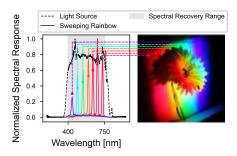
Figure 4. Temporal evolution of spectral illumination patterns of our system. Different narrow-band illuminations are projected to different locations of the scene, forming a sweeping rainbow strip pattern. Spectral characteristics of the broadband light source and reconstructed hyper-spectral imaging range are also elaborated.
