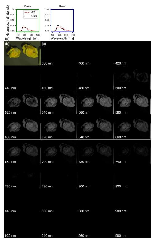
Figure 19. Evaluation of metameric samples of fake (left) and real (right) yellow roses. (a) Spectra of metameric samples against ground truth measurements, highlighting the system's ability to capture subtle spectral differences. (b) The reconstructed hyperspectral image in sRGB. (c) Estimated hyperspectral images.
