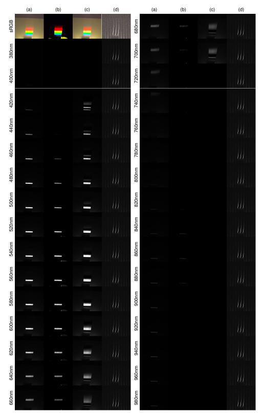
Figure 14. The full hyperspectral reconstruction results for examples in Fig. 5. Comparative analysis of spectral reconstruction on a high-frequency rainbow pattern. Compared methods include (a) ground truth, (b) ours, (c) basis-based method, and (d) bandwidth-matched frame-based method.
