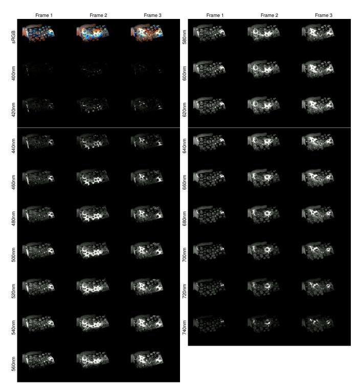
Figure 20. Real-time hyperspectral imaging on a moving iridescent sticker paper. Top-left: Three consecutive estimated hyperspectral images rendered in sRGB. Remaining panels: Corresponding estimated hyperspectral images (380-780nm, sampled at 20nm intervals).
