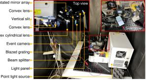
Figure 10. System prototype (corresponding to Fig. 1(a)).
