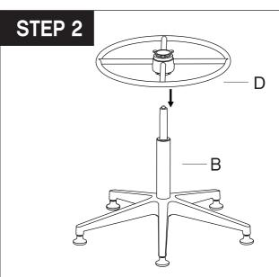
Please insert the Footring (D) onto the Seat Post (B), and adjust the Footring (D) to the desired height. Turn clockwise to tighten, and turn counter-clockwise to loosen.
