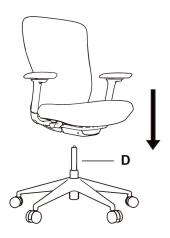
Now turn the assembled seat upright and locate the center hole of the Mechanism over the Seat Post. Push down firmly until the connection is secure.
