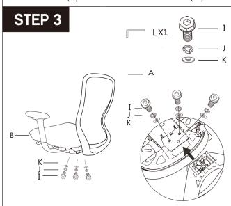
Please be careful to use the correct Back screws ( I ). Slide one spring Washer (J) and then a Flat washer (K) over each Backrest Screw (I). Tighten securely using the enclosed Allen Wrench (L).
