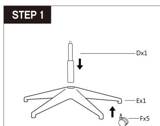
Press the Casters (F) into the holes at the end of each leg of the Base (E).
