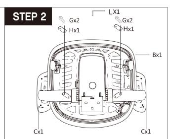
Please be careful to use the correct Arm Screws (G), For easy assembly, place the Seat (B) face down on a flat surface. Attach Armrest (C) to the seat (B) as shown using 3 Arm Screw (G) on each arm. Tighten the bolts securely with the enclosed Allen Wrench (L).
