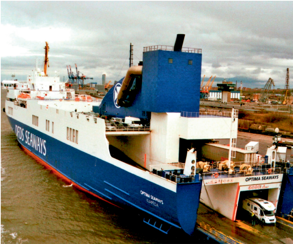
454 OPTIMA SEAWAYS seen on 30.03.2015 at Klaipeda after installation of a scrubber unit. Notice the bulky structure around the funnel.
