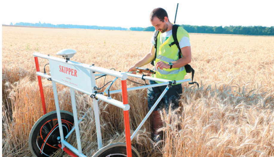
Magnetic tomography inspection of pipelines in conjunction with specialist contractor Skipper.
